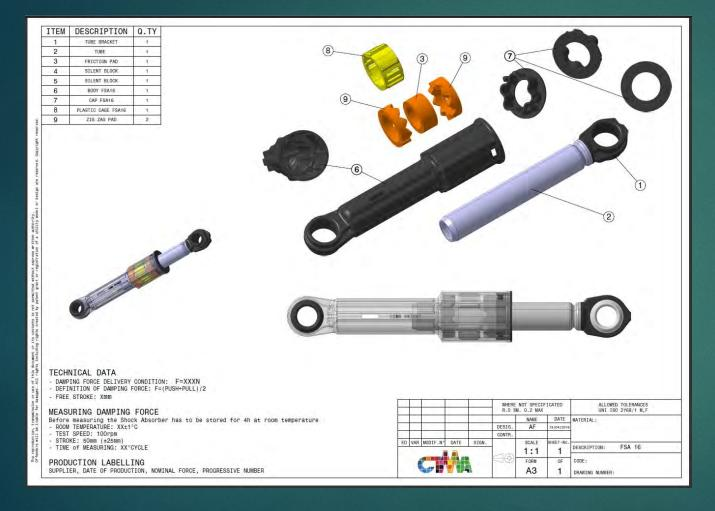
We have changed the design of all plastic components obtaining a reducing of the weight and an improving of the geometry.
